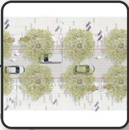
Typical Section D: Pedestrian comfort zone on west side and shared zone on east side
